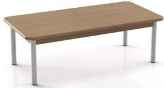
**Bases - 4 Pt** Constructed of high carbon content cold rolled seam welded flash controlled steel tubing. Offered in 1 7/8 in. O.D. 14 Gauge tube. Legs are welded to table support brackets that intern are connected to both the table top and the wood side supports.
