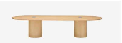
Bases - DR, DDR,Drum bases are made using a 3/4" thick particleboard frame wrapped with 1/4" thick plywood,HDRcovered and bonded with a water-based glue to a 1/16" high-pressure laminate sheet or laid up<br/>veneer on top.
