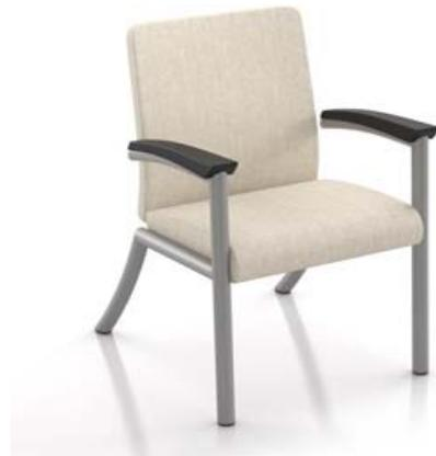
**Frame Construction** A combination of 14 & 16 gauge 1 3/4" O.D. welded steel tube is used to construct a frame free of crimping on all bends. Welds at joints are ground smooth to ensure safe use and to provide a uniform transition. Stretcher bars welded to the frame provide seat support. All connections are metal to metal. The frame is comes with an integrated steel arm.
