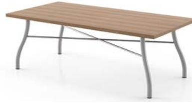
**Bases - 4 Pt** Constructed of high carbon content cold rolled seam welded flash controlled steel tubing free of crimping on all bends. Offered in 1 1/4 in. O.D. 14 Gauge tube. Welds at joints are ground smooth to ensure safe use and to provide a uniform transition. Legs are welded to table support brackets that intern are connected to both the table.
