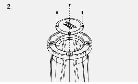
Add weighted ballasts into cavity and replace and ballast door and panel screws. Tighten panel screws 3-5 turns past finger tight.
