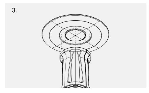
Align the table base to the center of the table top. Check fitment and make any necessary adjustments.
