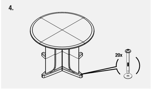
Flip table top over. Place assembled legs into pocket on bottom side of table top. Insert and tighten each table top screw 3-5 turns past finger tight.
