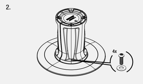
Insert and tighten each table top screw and washer 3-5 turns past finger tight.
