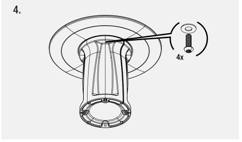
Insert and tighten each table top screw and washer 3-5 turns past finger tight.
