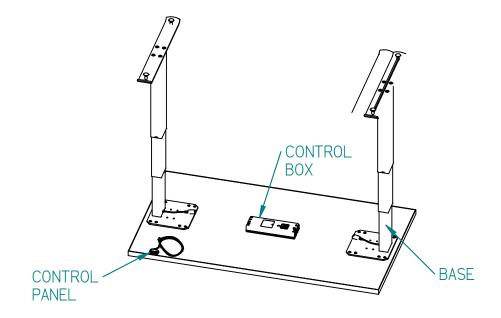
**NOTE:** CONTROL PANEL and BASES must be connected to CONTROL BOX first, before connecting to power.
