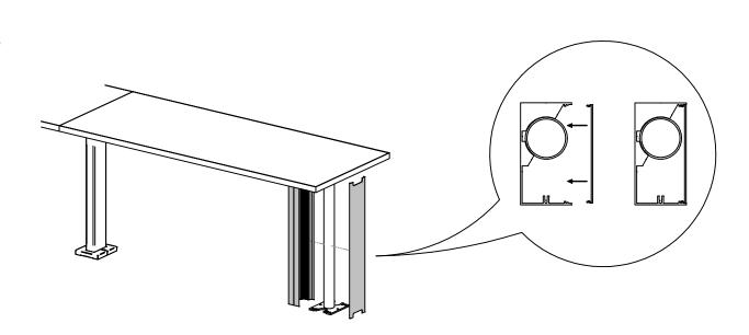
FOR POST LEGS WITH <u>RECTANGULAR VERTICAL WIRE MANAGER</u>: attach Rectangular Vertical Wire Managers first.
