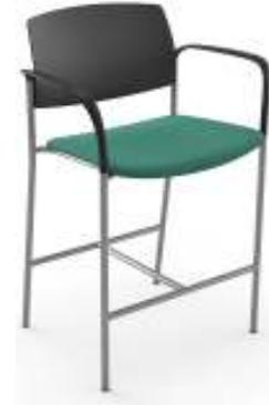
**Frame Construction - Stools** Constructed of high carbon content cold rolled seam welded flash controlled steel tubing free of crimping on all bends. Offered in 7/8" O.D. 14 Gauge tube. Stretcher bars are welded to the frame to provide seat support. All connections are metal to metal. A combination of brazing and MIG welding is used on all exposed welds.
