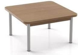
**Bases - 4 Pt** Constructed of high carbon content cold rolled seam welded flash controlled steel tubing. Offered in 1 7/8 in. O.D. 14 Gauge tube. Legs are welded to table support brackets that intern are connected to both the table top and the wood side supports.
